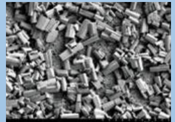
Wax crystals in Shoco Premium Diesel Fuel.
